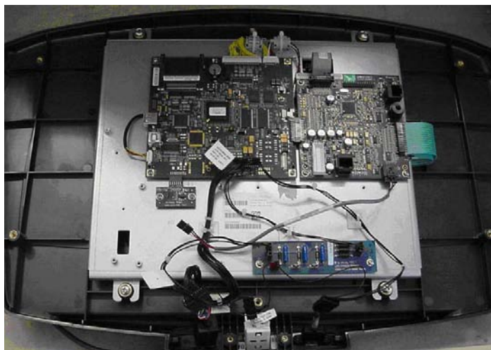
This picture shows the printed circuit boards mounted in the production 7-inch LCD treadmill console.
