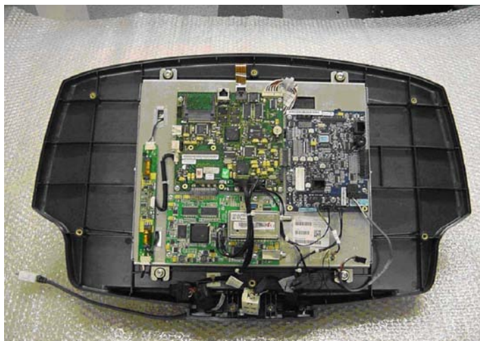
This picture shows the printed circuit boards used in the production 15-inch LCD treadmill console.
